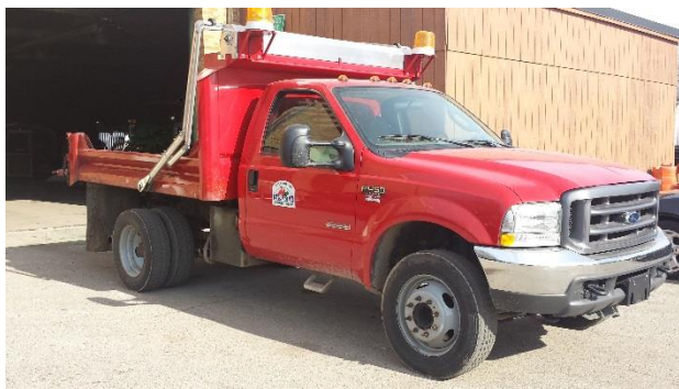
7 – Ford Super Duty 1 Ton Dump Truck (2004) Department: DPW Miles: 48,225 Hours: 4,798 Miles in Last Year: 2,621 Hours in Last Year: 263 Condition: Good
